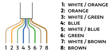
Detail C Ethernet Cable Wiring
